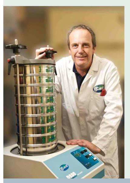
There are three essential characteristics to look for in a good test sieve shaker. It should generate an effective sieving action for tests to reach an ultimate end point. The end point should be reached in the shortest possible time. The results achieved should be reproducible.
