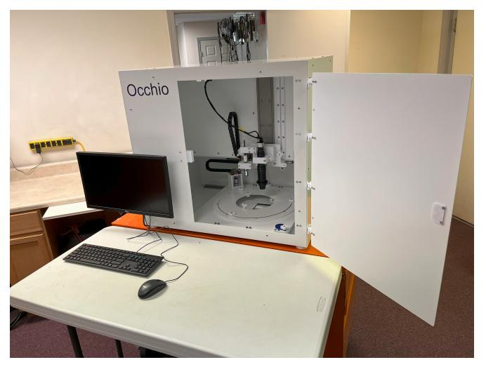
Newly redesigned chassis is smaller than the previous model. The computer is also mounted in the side of the instrument. The monitor may be mounted on the front of the instrument if desired using the monitor mount hardware.
