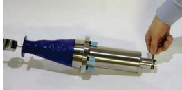
5. Slide out the inner shaft assembly.
