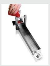
A measured sample up to 100 ml is placed in the reservoir behind the gate.
