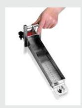
released gate by pressing the lock release lever - the spring action ensures it opens instantaneously.
