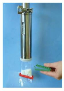
Quick Clips provide an instant removable seal for use with layflat tubing or bags. Ideal for use in ATEX rated areas where a heat sealer can not be used.
