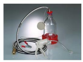
Sampler especially developed for sampling flammable liquids of Hazard Category AI (VbF, e.g. fuel). Glass bottle and hose are connected in such a way that they conduct electricity and are earthed via an earthing cable.
