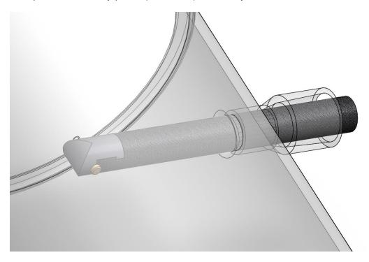
The agglomeration accessory is fitted into the GL32 port on the glass tub. The top cap must be removed, and the agglomeration accessory inserted from the inside of the tub.
