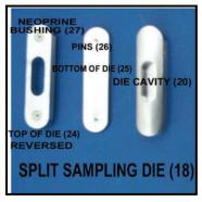
Each Split Sample Die is made of two 316 SS sections snapped together by hand to form the die. The upper section has the sampling cavity and the lower section is blank. The split design allows ejection of the compacted tablet. These dies fit in Models 675 1230A (Single Style), 675 GIA, 675 1230B (Double Style), 675 1230C (Triple Style), and cover a sample size range of 0.1 cc to 3.0 cc in increments of 0.1cc.
