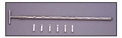
Standard single-sample design. 0.875" in diameter. One unit-dose sample is obtained at each sample port. The bottom most port starts at 1.5" from the tip. 40 different sizes of sample dies (0.1cc to 4.0cc in increments of 0.1cc) and 30 different sizes of split sample dies (0.1cc to 3.0cc in increments of 0.1cc) fit in this sampler. Stock sizes are 1ft with 5 ports, 2ft with 10 ports, 3ft with 6 ports, 4ft with 8 ports, 5ft with 10 ports and 6ft with 12 ports.
