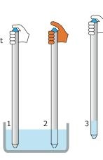
The deeper the sampler is pushed into the liquid the larger the sample volume
