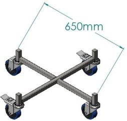
Method of Construction: Frame - welded
