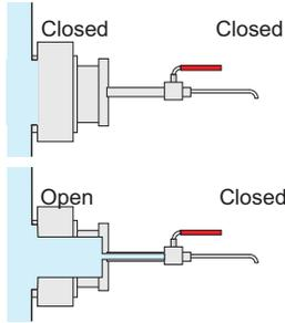
1. Connect the Road Tanker Sampling Valve to the main discharge valve on the road tanker.
