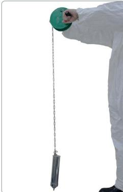
\* Make sure the sampler is properly earthed (grounded) use the Ex Hand Reel (5070D-05) and Copper cable (5070C)
