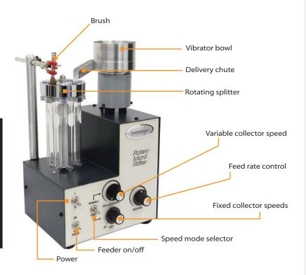
The Rotary Micro Riffler™ easily and automatically divides samples into eight (8) smaller representative samples for analysis. By repetitive divisions of the collected smaller samples, the desired final sample size can be easily obtained.
