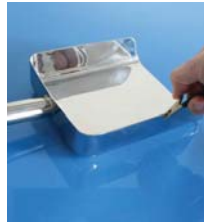
2. Attach Lead on item that is to be etched
