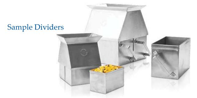
These hand held sample dividers will subdivide material samples into two smaller portions by a single pass or further subdivisions can be attained by multiple passes. The important feature of Endecotts sample dividers is that each subdivision retains the characteristics of the original sample. Based on the recommendations of BS 5309 and BS 3406/1. Produced in stainless steel with slot widths of either 6.35 mm (1/4") or 12.7 mm (1/2").
