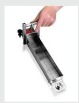
The gate is released by pressing the lock release lever - the spring action ensures it opens instantaneously.
