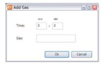
the bottom of the screen to add these values. Once the button has been clicked a screen will popup showing the current time of the roast. If the user types in a value, then that value will be entered corresponding to the time that is displayed.
