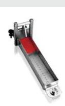
As the fluid flows down the instrument its progress can be accurately measured using the graduated scale. By comparing the flow rate to specified time periods the physical properties of the sample can be calculated.
